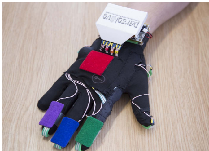
Figure 1. ParsGlove is an innovative wearable interface which is designed and developed to capture the human hands ergonomics and to provide this information as an interactive input both for the game and the application.
